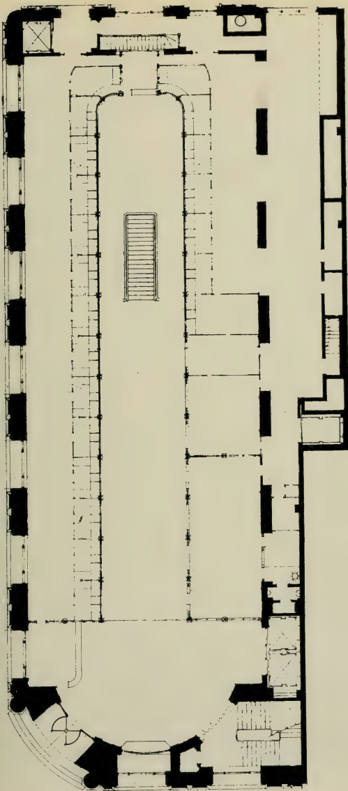
Main Floor Plan, Bank of Italy, San Francisco (Plan reproduced at scale of 1 inch = 24 feet)
